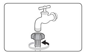
If using a screw type of water tap, connect the water hose to the water tap as shown.
