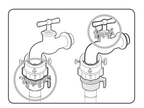
**8.** Open the water tap and check if there are any leaks around the connection areas. If there are water leaks, repeat the steps above.
