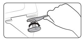
**3.** When levelling is complete, tighten the nuts using the spanner.
