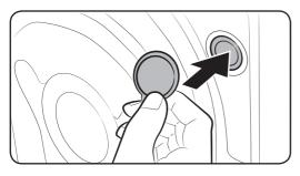
**2.** Fill the holes with the supplied plastic bolt caps.
