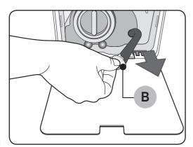
3. Put an empty, spacious container around the cover, and stretch the emergency drain tube to the container while holding the tube cap (B).
