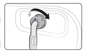
**7.** Connect the other end of the water supply hose to the inlet valve on the back of the washing machine. Turn the hose clockwise to tighten.
