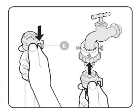
**6.** While holding down part (E), connect the water supply hose to the adaptor. Then, release part (E). The hose fits into the adaptor with a clicking sound.
